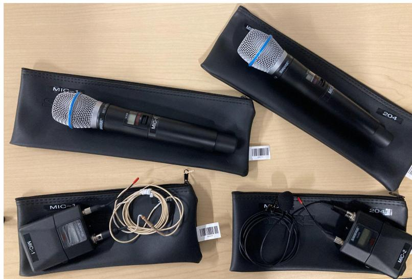
**Note:** There is 1 handheld and 1 lavalier/lapel microphone per microphone channel in each room. If you are using both a lavalier/lapel and a handheld mic, you must make sure that they do not have the same microphone number. So if you are using lavalier Mic-1 you must use handheld Mic-2 to use both at the same time.
